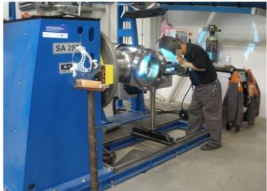
Control system: KSK –SA 207 –2 controlled axes Positioner capacity 3,500kg with support Turning diameter 1 800 mm The length of the weld. Workpieces max. 1 350 mm
