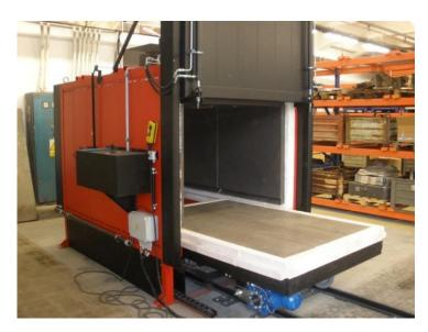
There are available chamber electric furnaces to provide pre-heat process and heat treatment. The furnaces are equipped with digital controls which allow controlling of heat. Digital or paper record belong to the furnaces equipment of the heat treatment. Local preheating and other technological heating are ensured by gas burners.
