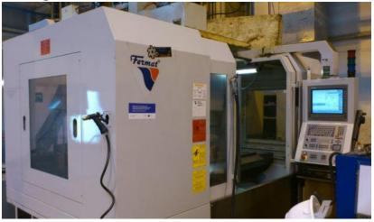
Horizontal Boring Machine - WFT 13 CNC
