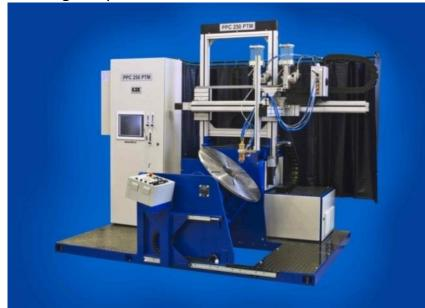
Control system: KSK –PPC 250 PTM –5 controlled axes Positioner capacity 600 kg Max. turning diameter 1 200 mm The length of welded-on workpiece max. 600 mm 1 200 mm to diameter 150 mm
